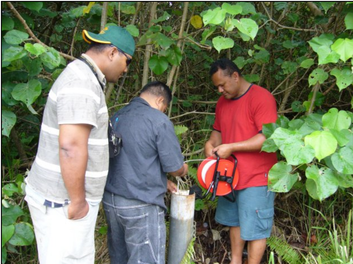
Figure 23 Measuring the thickness of the freshwater lens at SMB3 in the Mataki'eua wellfield using the Solinst TLC dipmeter
