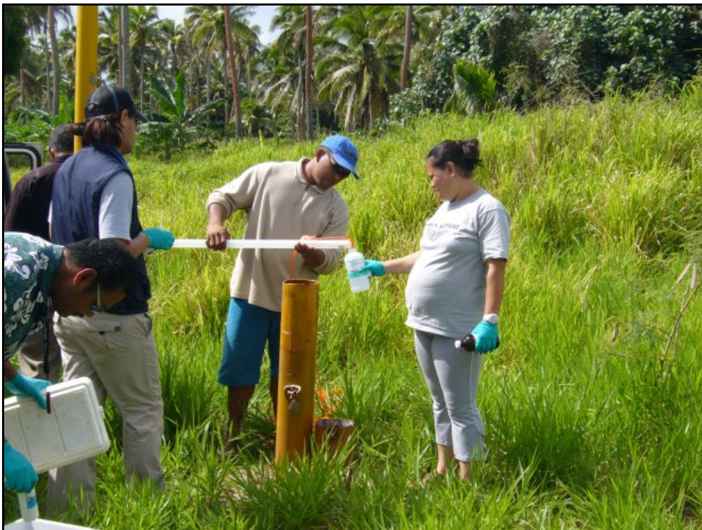
Figure 12 Multi-agency monitoring team collecting groundwater samples from a bore near the Tapuhia waste facility for the WA
