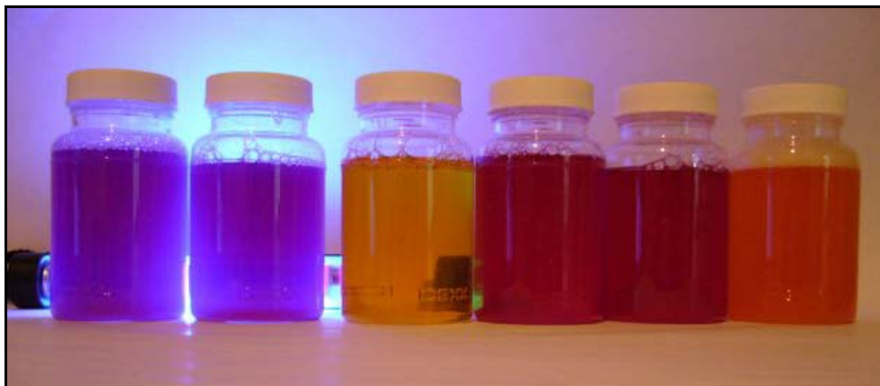
Figure 28 Results of Colisure tests for the presence of E. coli (fluorescent blue), total coliforms (red), or their absence (yellow)
