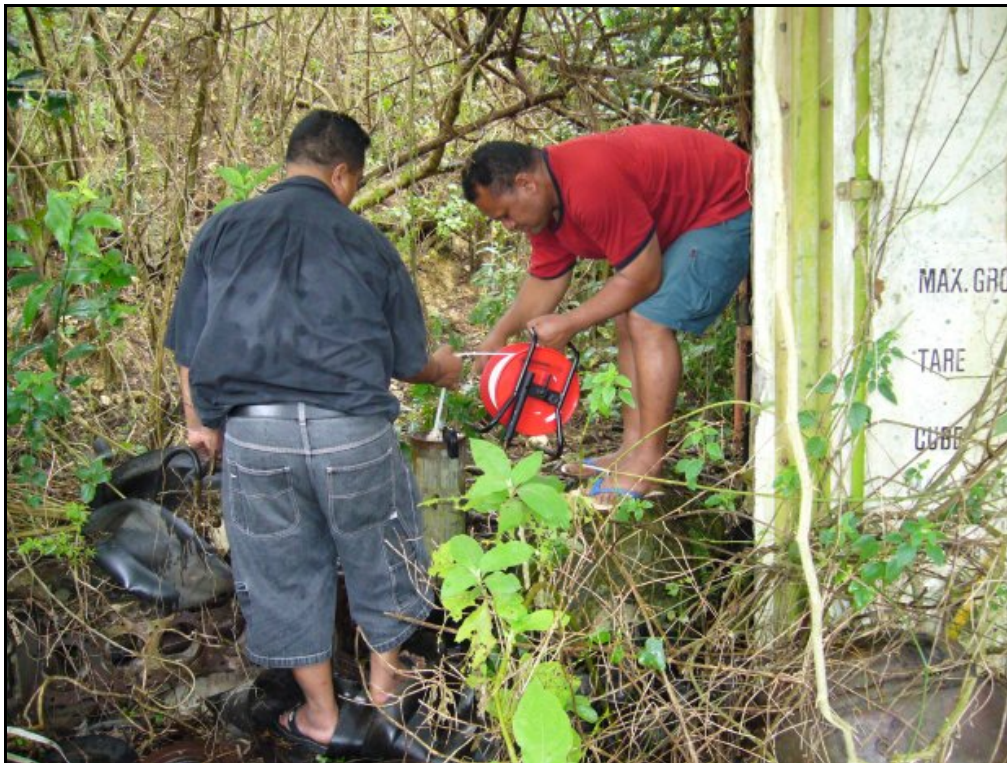
Figure 166 Salinity monitoring borehole SMB6 in the middle of industrial refuse in the Kahoua Quarry
