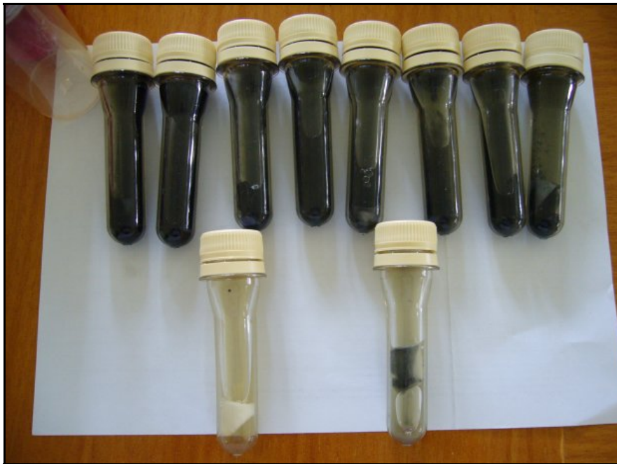
Figure 29 H 2 S paper strip test for the presence of bacteria. Where the paper strip and water are black there is the very high risk of faecal contamination, partial black means some risk of contamination while the clear sample indicates no risk.
