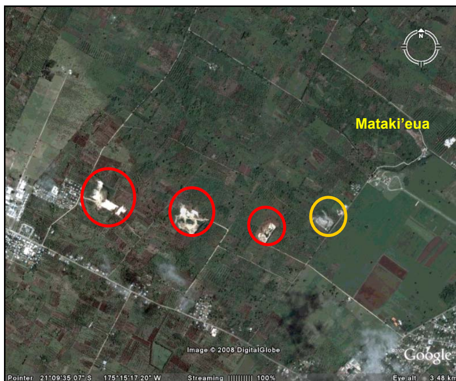
Figure 158 Quarries close to the Mataki'eua/Tongamai wellfield. Active quarries at Kahoua, Hauloto and Tafolo (left to right) are circled in red, an inactive or partially active quarry in yellow. The closest quarry is 0.75 km from the nearest TWB well (Google Earth).
