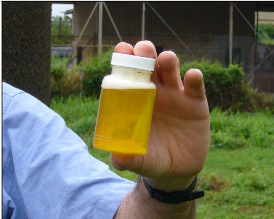
Figure 27 Testing a rainwater sample for faecal contamination. The Colisure substrate has just been added.
