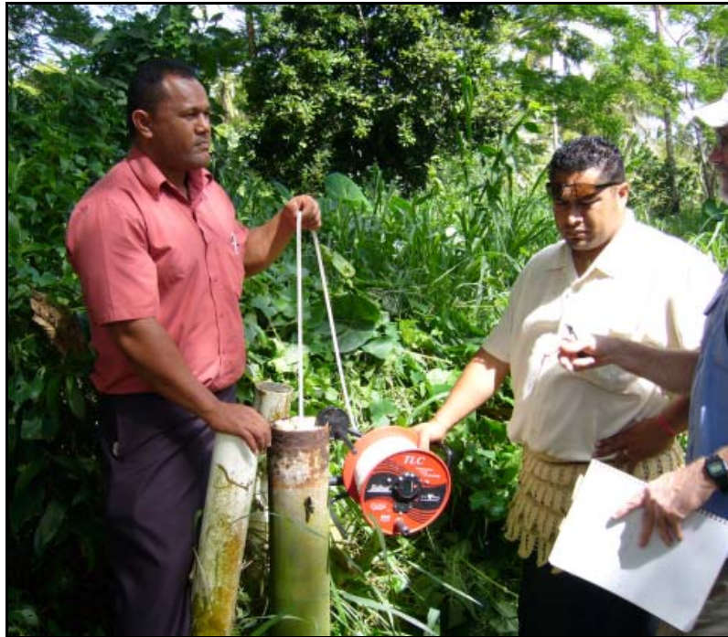
Figure 182 Measuring SMB7 salinity profile using the Solinst meter bought under HYCOS
