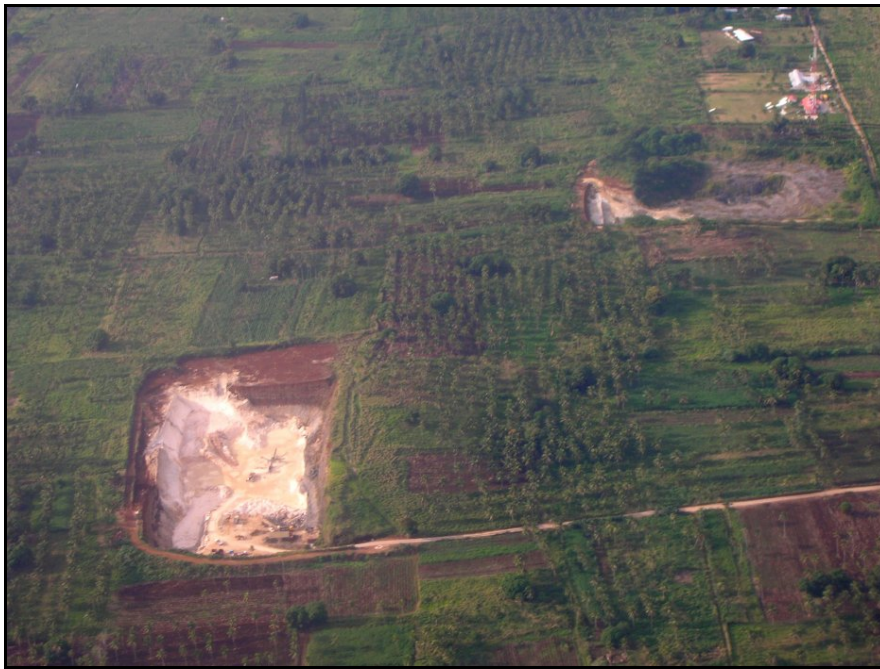
Figure 159 Aerial view of the Tafolo quarry close to water wells in Mataki'eua. The quarry on the right is within 0.75 km of the nearest well, while that at Tafolo on the left is within 1.1 km. Note the exposed water table in the lower left of the Talofa quarry.
