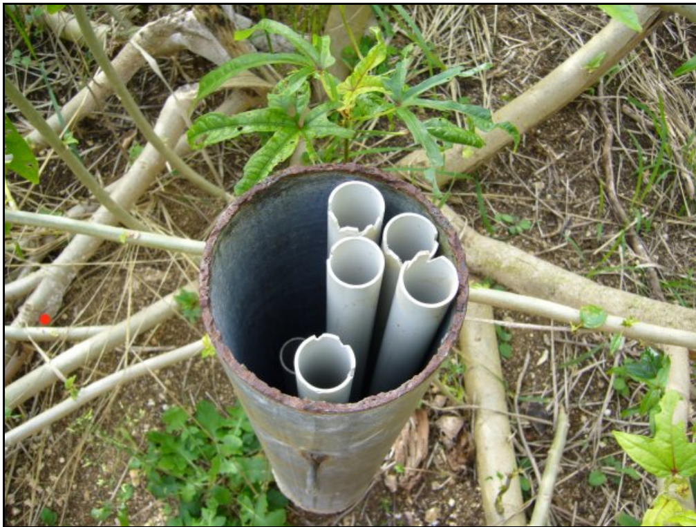
Figure 21 SMB2 showing the tubes for sampling different depths through and beneath the freshwater lens in the Mataki'eua/Tongamai wellfield close to TWB pumping well 105
